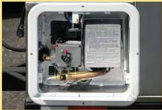
Combination 6 gallon gas/electric hot water heater. Use either or both at the same time for reduced recovery time.
