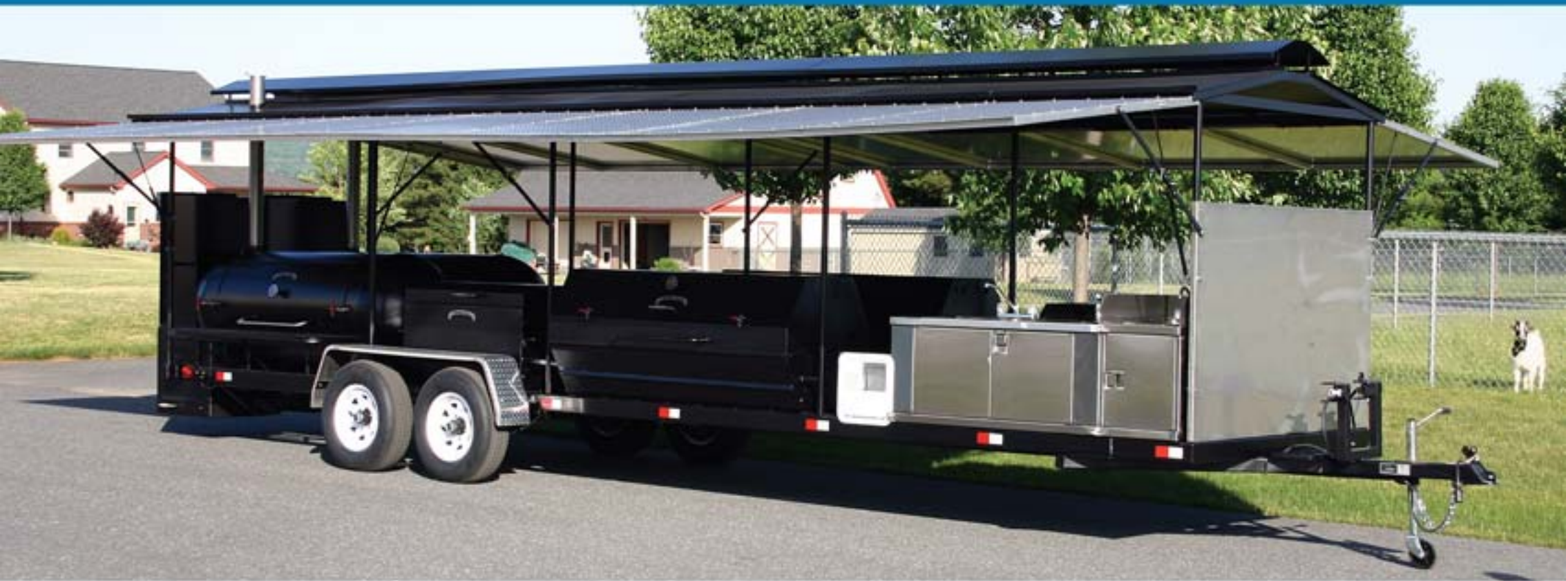
Shown with full length hinged roof that folds down and locks for transport.
